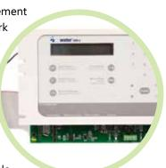
IrriCare IRP communicates over cellular network with specially designed, dedicated hardware devices called 'IrriConnect Master'. IrriConnect Master further communicates through RF with filed remote terminal units (RTU) called 'IrriConnect PRO'.
