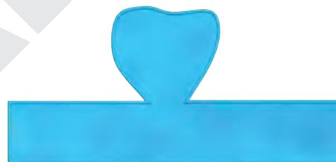
Over Pressure - Poor Weld
