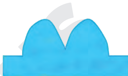
Low Pressure - Poor Weld
