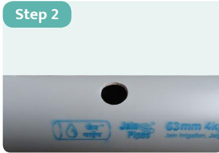
Deburr the hole carefully. Check that no sharp corners are present.
